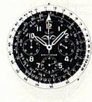
Solution: Set 271/2 gallons on the white disc opposite 145 minutes on the black disc. Opposite the "hour index" disc). read the rate of consumption which is 11.3 gallons per hour.
