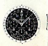
Solution: On the white disc set 156 opposite the hour index on the black scale. On the outer black scale opposite 486 on the white scale read 187 minutes (or 3 hours and 7 minutes on the inner black scale).
