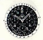
Solution: Set 30 (= 300) on the white disc opposite the "unit index" (the numeral "10") on the black disc. Now opposite 34 on the black disc read 10,200 feet on the white disc.
