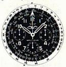
Solution: Opposite the "hour index" set 11.5 on the white disc. Then, opposite 31/2 hours on inner black scale (210 minutes on outer black scale) on the white scale read 41 gallons.
