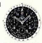
Solution: Move the white dial until 104 on the white scale is set opposite 35 on the black scale. Opposite the hour index (the arrow marked "MPH" directly over the hour 12) read 178 miles per hour on the white scale.
